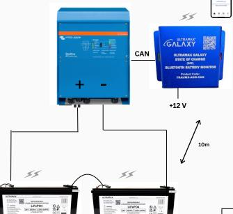
The Bluetooth aggregator can collect data on State of Charge & other parameters such as current, voltage, temperature and alarms from 1 to 10 parallel or 4 in series connected batteries via Bluetooth.
