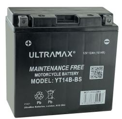
Factory Activated.sealed Ultramax motorcycle batteries ,with acid being completely absorbed into glass mat separators which are sandwiched between the lead plates, giving a sealed and maintenance free battery.
